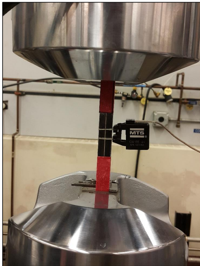
Figure 31. Specimen Setup on MTS 810 with extensometer installed
